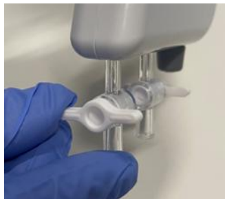
FIGURE 7: IN-FLOW AND OUT-FLOW IN CLOSED POSITION
