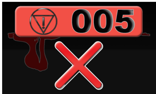
Figure 29: Minerva Disposable Handpiece Integrity Test Failure
