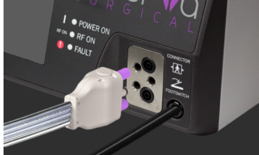
Figure 13: Connect Minerva Disposable Handpiece and Footswitch
