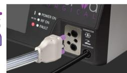
**CONNECT HANDPIECE & FOOTSWITCH** to the appropriate port on the front panel of the Minerva RF Controller.
