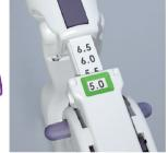
Press toggle switch to set the PFA Length using cavity length calculated in step 1.
