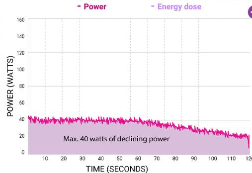
Software delivers a patient specific dose of thermal energy, which results in a uniform depth of ablation and complete tissue coverage (graph represents titration of power over the 2-minute treatment cycle)
